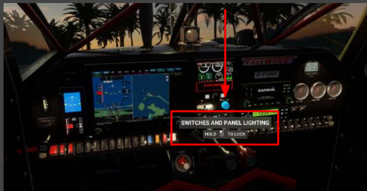
AVIONICS ON / PANEL LIGHTING ON / LAST IS DIMMABLE
