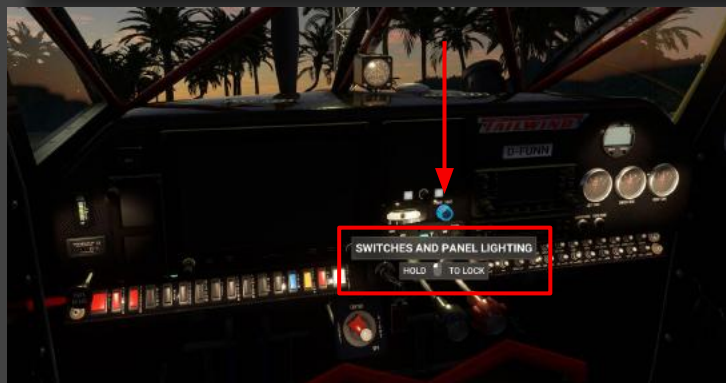
GLARESHIELD TYPE OVERHEAD LIGHTING FOR SWITCHES AND CIRCUIT BREAKERS
