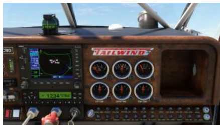
CONTROL-2 AVIONICS AND ENGINE INSTRUMENTS
