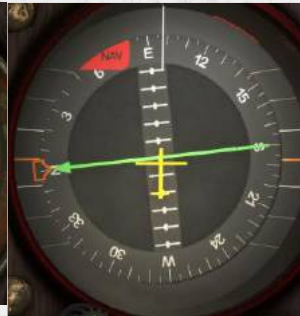
Horizontal Situation Indicator. With glideslope support and heading bug. Connected to NAV1.
