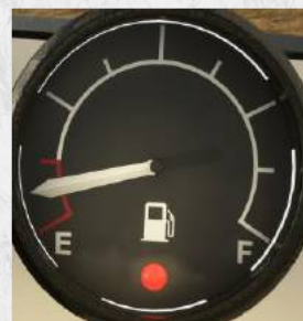
Fuel gauge with low fuel indicator light.
