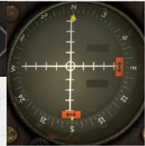
Course Deviation Indicator. With glideslope support. Connected to NAV2.
