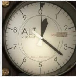
Altimeter with a QNH calibration knob.
