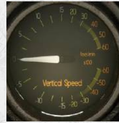
Vertical Speed indicator. Non-linear scale.
