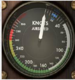
Airspeed – in knots. Taxi in the blue arc and flaps/gears extended not above the white arc.
