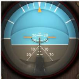
Attitude Indicator, with horizon level calibration.
