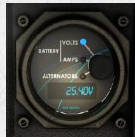
Battery & Alternators indicator. Already discussed.
