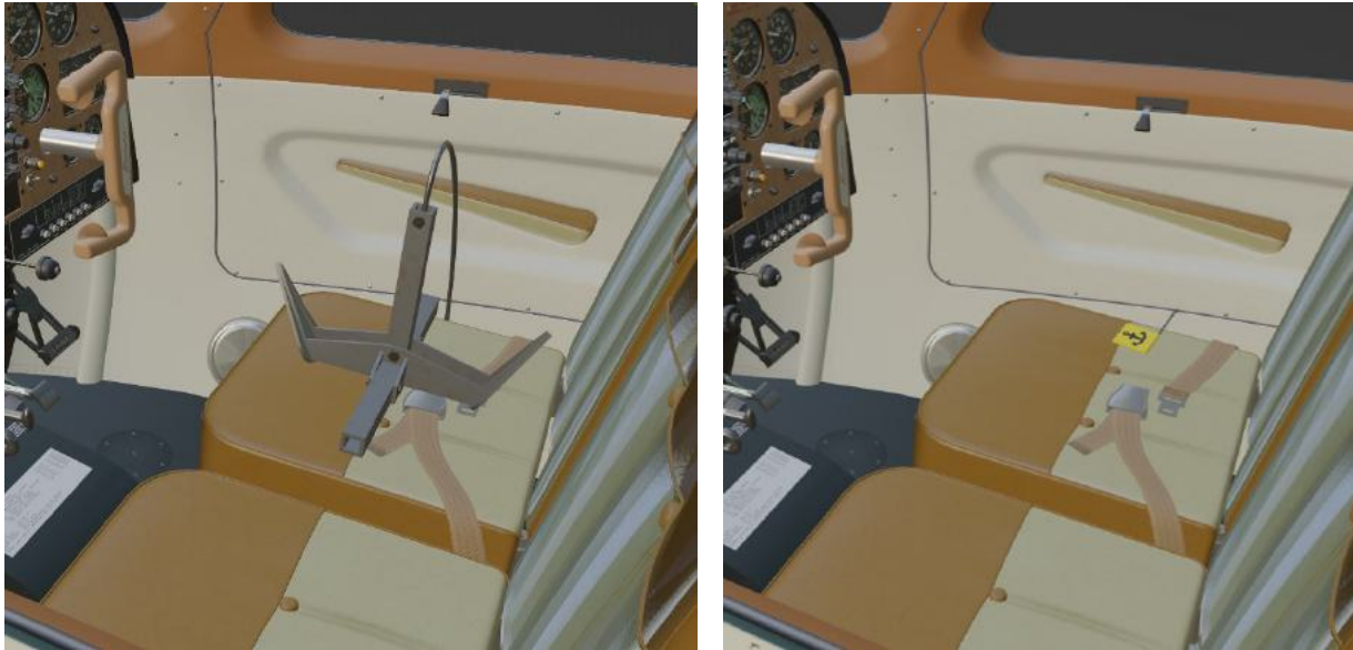
Figure I-6: Anchor Left: Available. Right: Deployed
