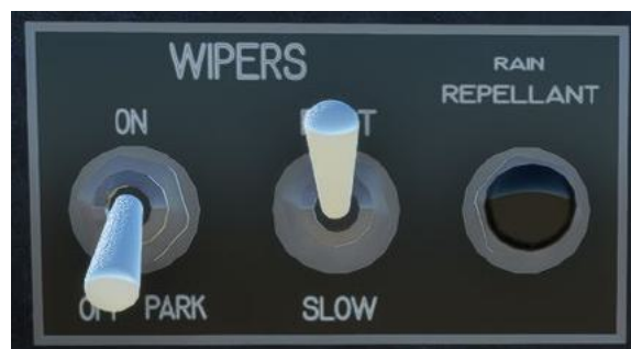
WIPER CONTROL PANEL (1P)
