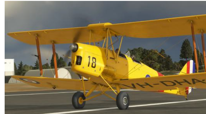
The take-off procedure is straightforward; the only thing to watch is the propeller torque pulling the nose to the right. Key Publishing
