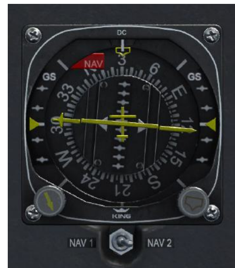
The HSI showing a selected heading of 30 degrees
