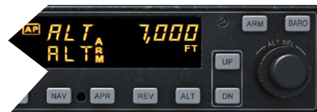
New altitude preselected with altitude select knobs; note ALT ARM is annunciated but autopilot remains holding previous altitude.
