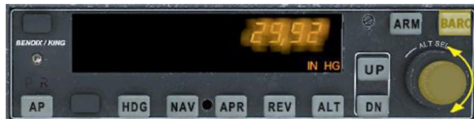
Adjusting the Barometric Setting
