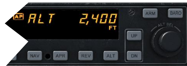
Altitude hold (ALT) mode active; autopilot holding at displayed altitude
