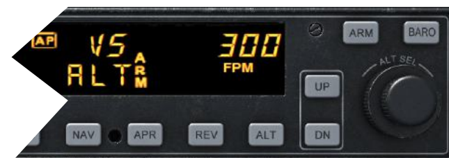
Clicking the [ALT] button engages vertical speed (VS) mode; a vertical speed of 300 fpm has been commanded by clicking on the [UP] button.
