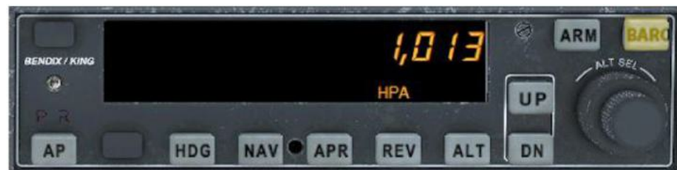
Toggling the Barometric display between IN HG and HPA
