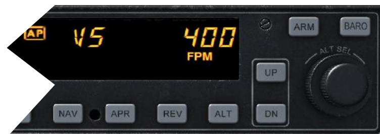
Vertical Speed (VS) mode active, with vertical speed value displayed
