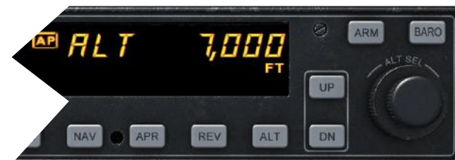
At the preselected altitude, the altitude is captured and altitude hold (ALT) mode is engaged. Note that the ALT ARM annunciation has extinguished.
