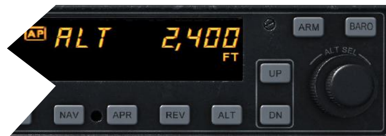
Altitude Hold (ALT) mode active, with reference altitude displayed
