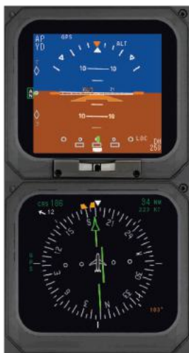
Electronic Attitude Director Indicator (EADI) & Electronic Horizontal Situation Indicator (EHSI)
