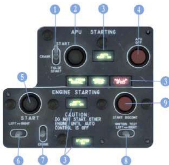
Figure 11-6. APU / ENGINES Starting Panel.
