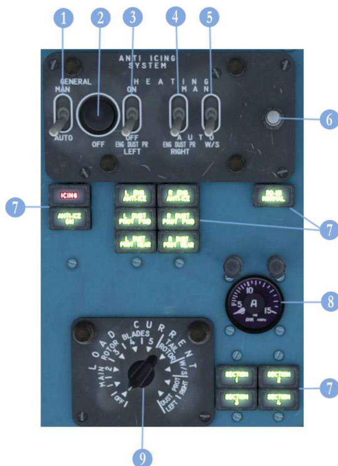
Figure 9-1. Anti-icing system panel.
