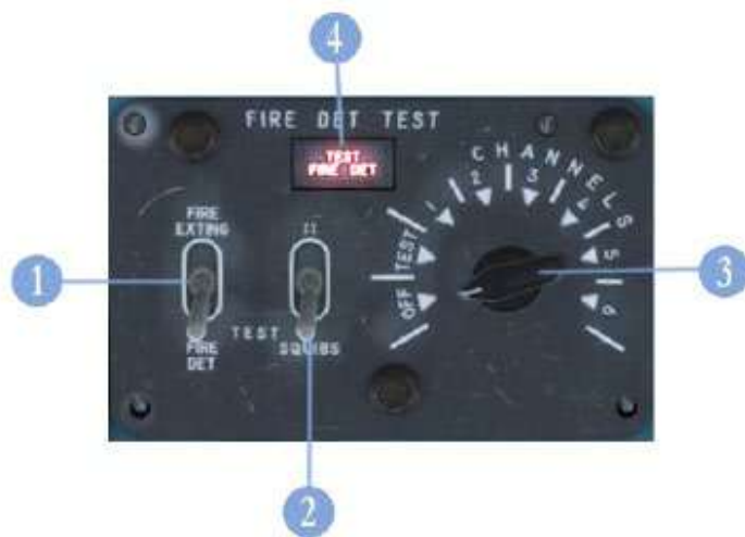
Figure 11-4. Fire Detection Test Panel.
