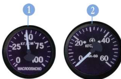
Figure 6-5. Air pressure gauges.
