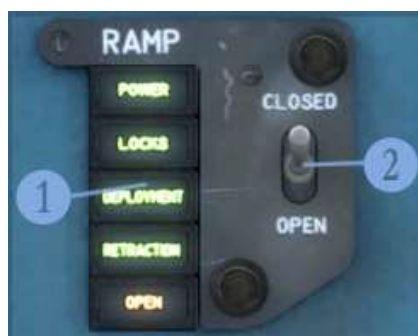
Figure 5-5. Ramp control panel.
