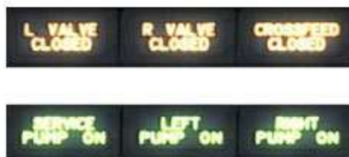
Figure 11-9. Annunciators Fuel Panel.
