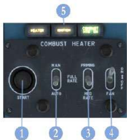
Figure 11-12. KO-50 Control Panel.
