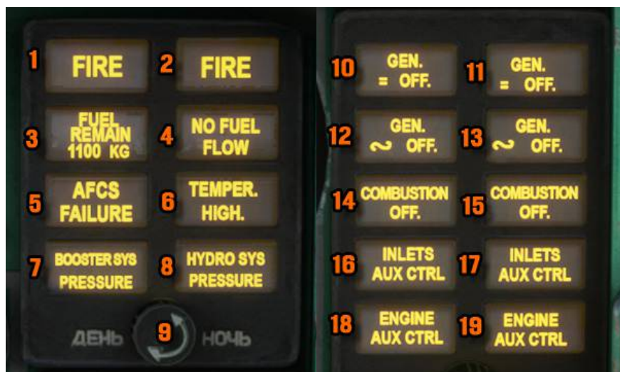
Warning panels 1 &amp; 2 (Pic. 6)
