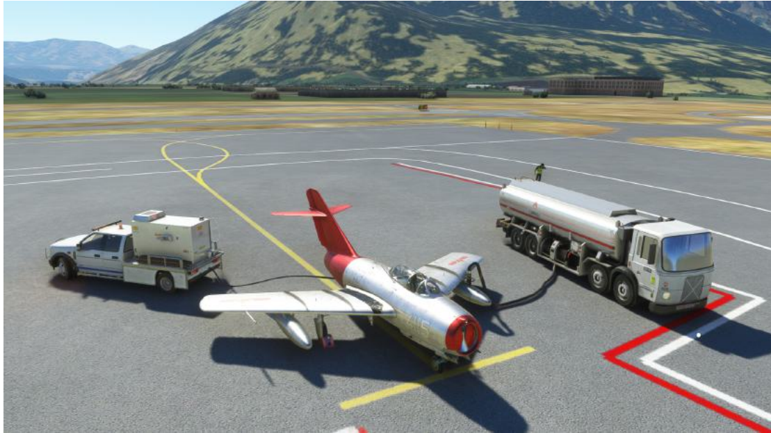
Fig 4-2 Fuel Truck and GPU connected on Ground
