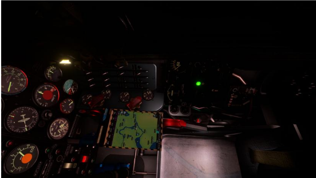
Fig. 0-14 Right Flood Light, AKR-7 Gauge Light, with Potentiometer Dimmer Controls
