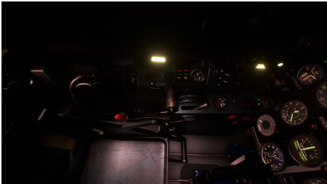
Fig. 0-15 Left Flood Light, Radio Display, with Potentiometer Dimmer Control
