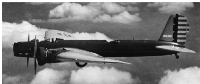
Top: Boeing YB-9. Even though seen here in the Olive Drab and Orange-Yellow colors of the USAAC, it was not accepted by the USAAC. However, it did greatly influence the design of the first modern airliner, Boeing's 247.
