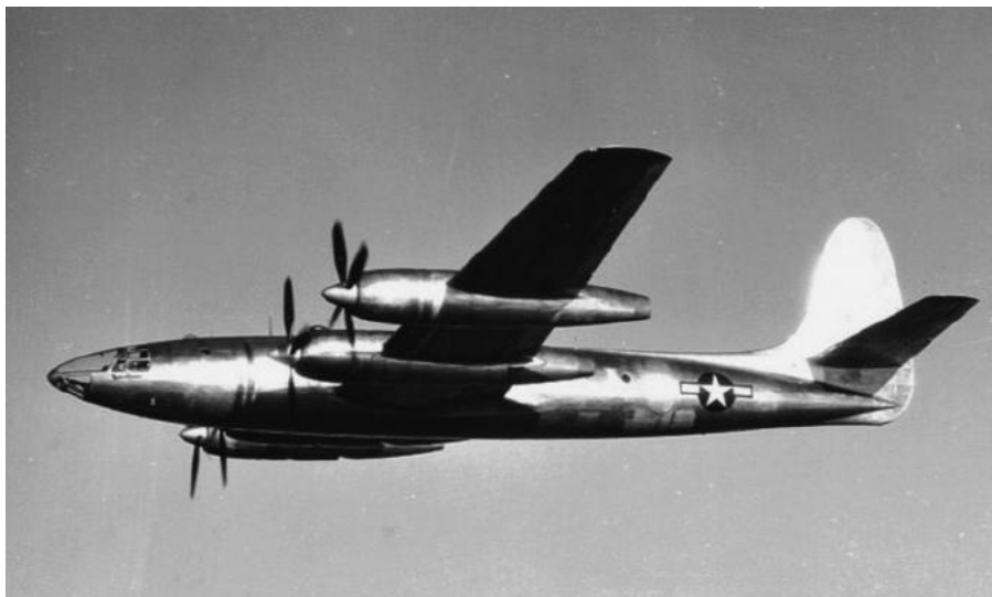
Republic "Rainbow" in the markings of the U. S. Army Air Force shortly before it became the independent U. S. Air Force. Proposed as a reconnaissance/aerial photography aircraft, "Rainbow" (USAAF designated XF-12, USAF designated XR-12) it had a top airspeed of over 470 mph at 45,000', making it one of the fastest piston-engine aeroplanes in the USAAF's inventory. However, the prototype's first problematic flight was not until 10 July 1947 when even faster jet-powered aircraft such as RB-47 were already being used for this mission. Accordingly, none were ordered and only two were built. Quel dommage, it certainly is a beauty.
