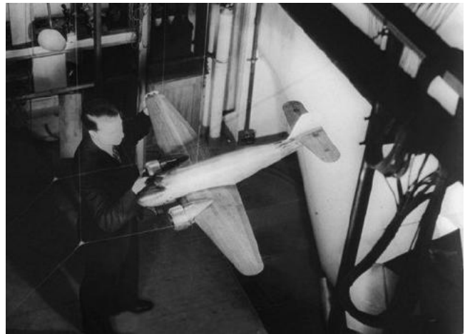
Clarence "Kelley" Johnson with the 55" scale wind tunnel model of the first, single tail design for Lockheed's Model 10 Electra.
