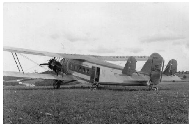
The Tri-Tail Boeing Model 80A-1. This was the latest advancement in airliner design in the late 1920's and early 1930's and would not be replaced until the revolutionary Boeing 247 in 1934. Photo circa 1930. It seems amazing that only thirteen years separate this aeroplane from the sleek and gracious all-metal Constellation.
