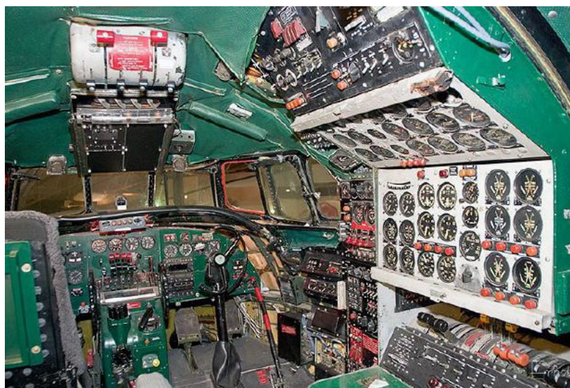
Got enough stuff? With the Co-Pilot's seat removed for clarity, the Flight Engineer's station on the right in the foreground and the Co-Pilot's switch panels on the right forward side of the cockpit are just a part of all that the crew of piston-engine airliners in the 1950's had to deal with. Jets are so much simpler. Note the plethora of engine controls under the main panel at the Flight Engineer's station.
