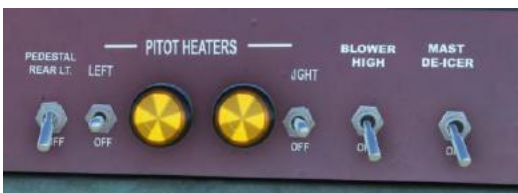
Pitot heater switches left and right are on the right side of copilot
