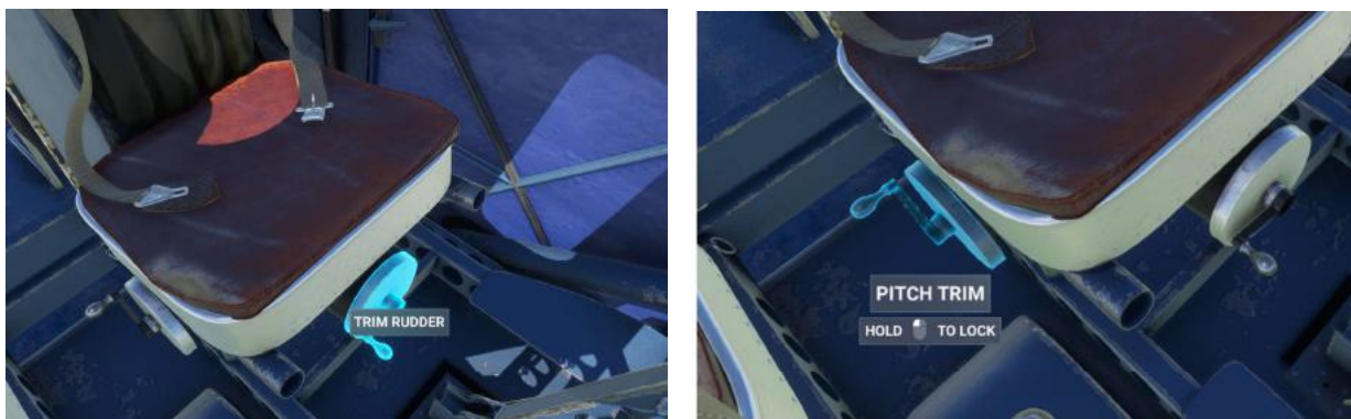
Rudder and pitch trim are located under the pilot seat
