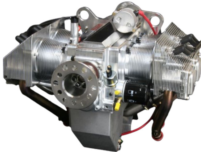
Figure 1-4 Jabiru J2200 4 Cylinder Engine
