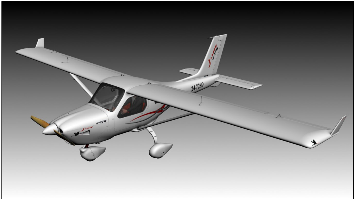
Figure 1-1 Jabiru J160/J170 General Arrangement
