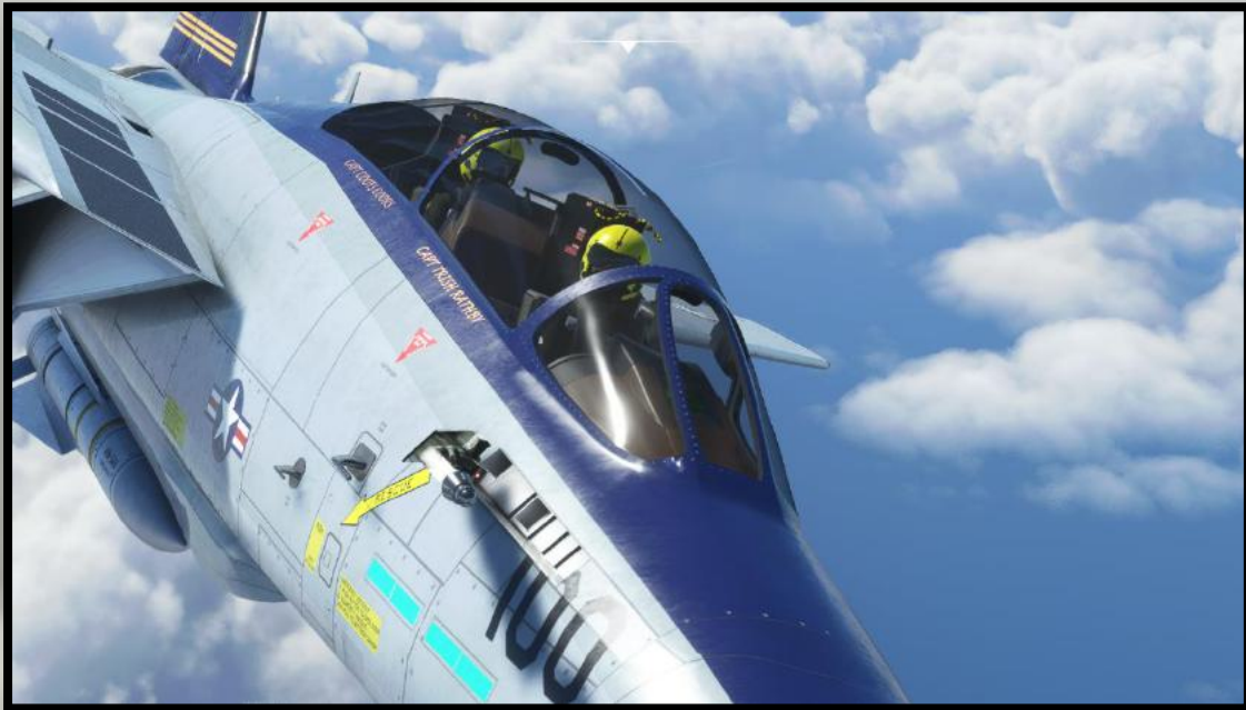
F-14A with fuel probe extended. A guide light automatically illuminates for night-refuelling purposes.
