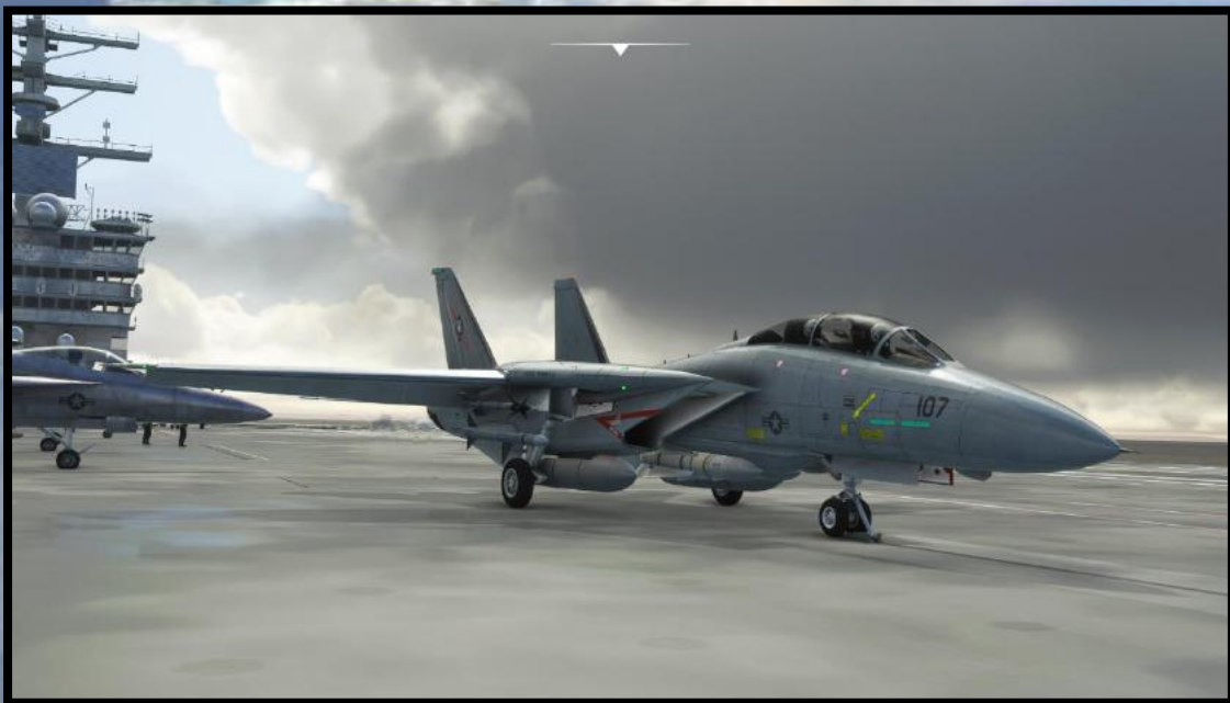
F-14A Tomcat "crouching" over the catapult shuttle prior to launch.
