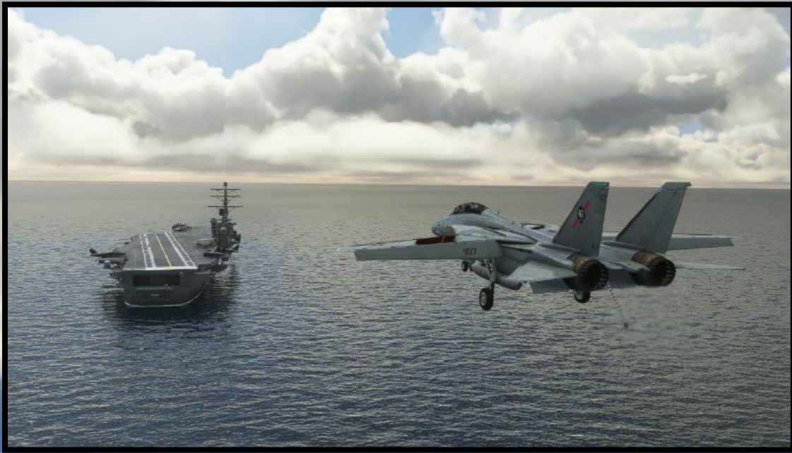
F-14A "in the groove" astern the carrier, lined up for landing.
