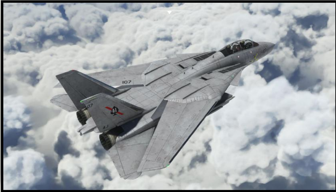
F-14A at supersonic airspeeds, with glove vanes extended.
