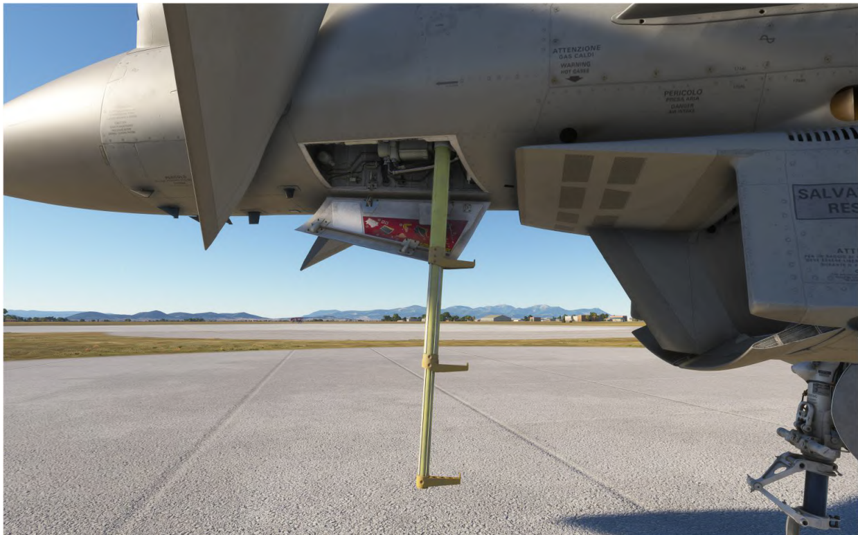
Cockpit Access Ladder (extended)
