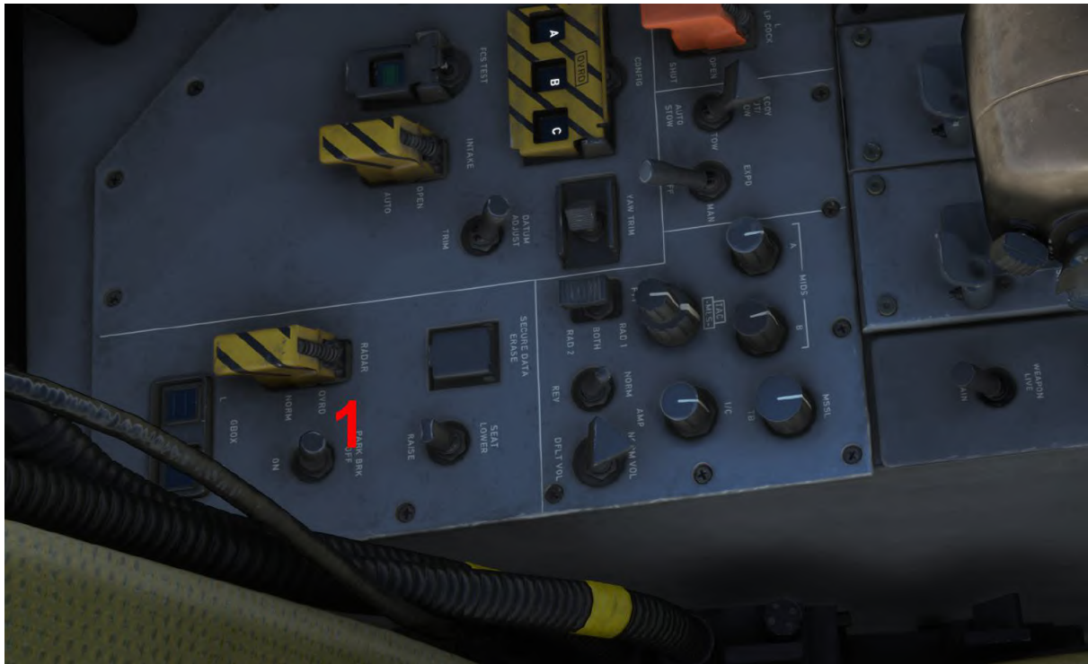
PARKING BRAKE CONTROL (Left console)
