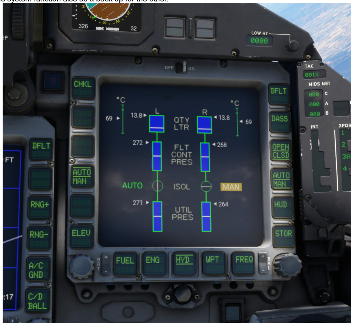
HYDRAULIC SYSTEM FORMAT
