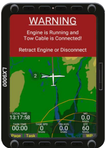
Tow Cable Unsafe Warning
