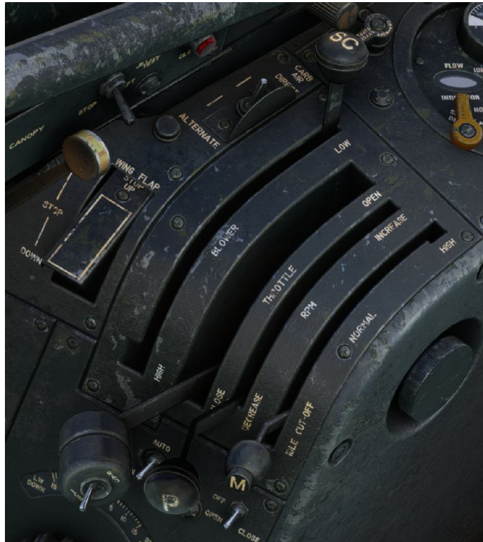
From Left to Right: Blower, Throttle, Propeller, Mixture
