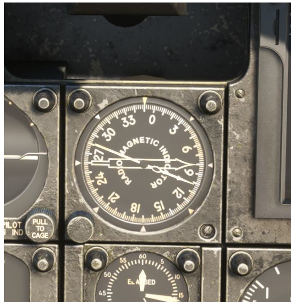
Small Needle displaying bearing to ADF.
