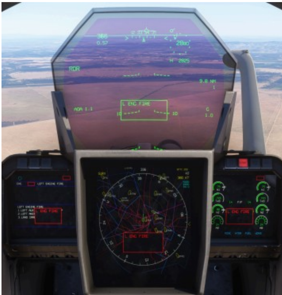
Red alarm displayed on main avionics screens
