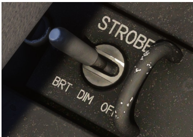
Strobe lights switch
