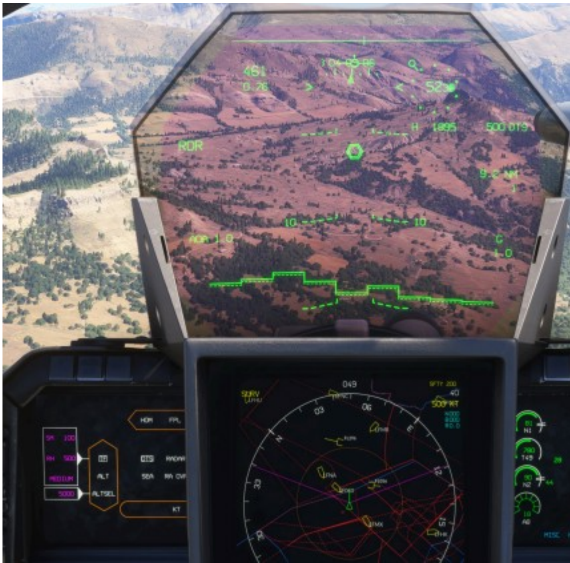
Terrain following selected but not controlled by the autopilot
