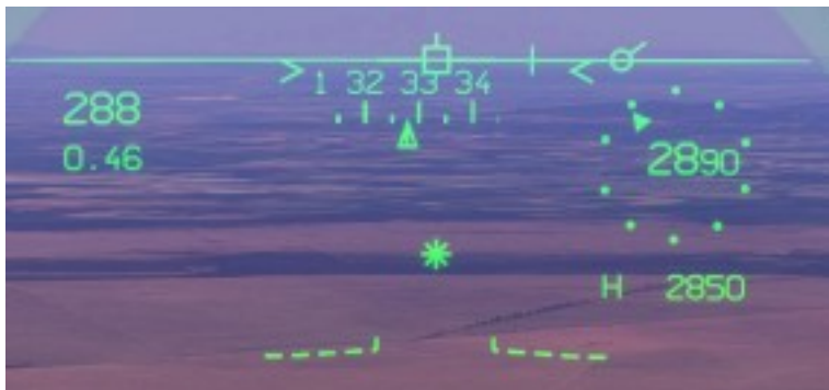
Asterisk indicating a pitch-down trajectory commanded by the flight director
