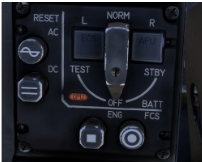
Indicator confirming that GPU is providing electricity
