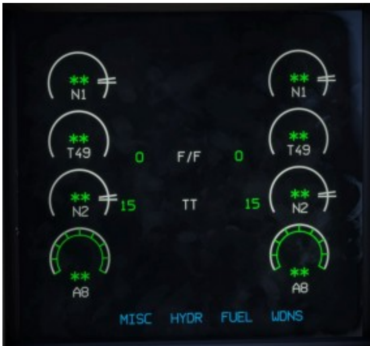
Display with the engine control units unpowered
