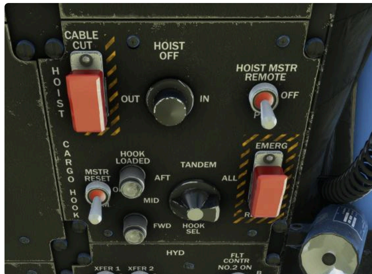
Overhead Panel - CARGO HOOK Panel. Note HOOK MODE SEL is set to MID
