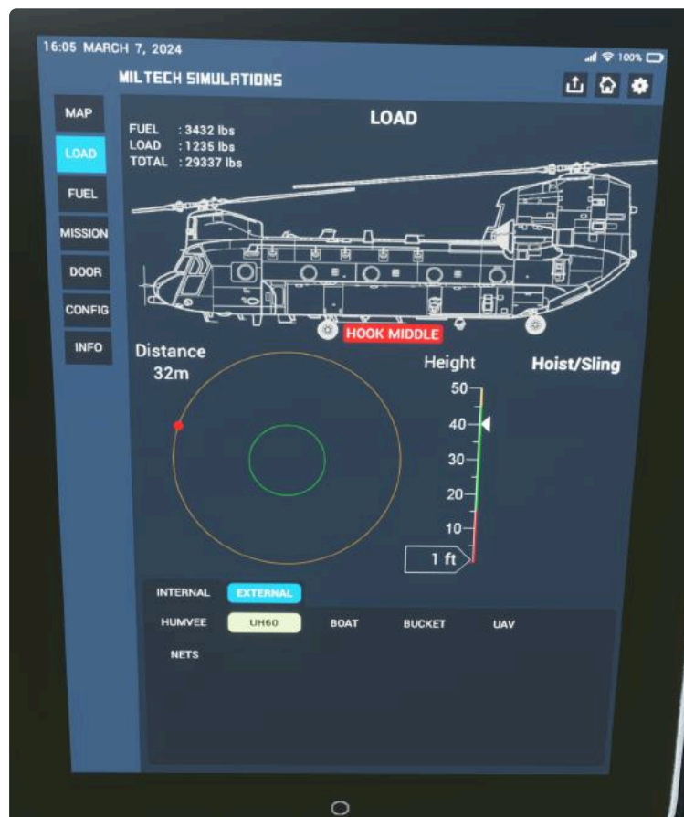
UH60 Load Selected. Note Red Blinking message to "Set Hook Mode to MIDDLE"
