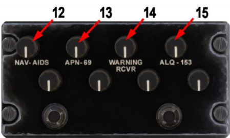
TYPICAL AUXILIARY MIXER SWITCHES FOR THE PILOT, COPILOT, INSTRUCTOR PILOT, RADAR NAVIGATOR, NAVIGATOR, INSTRUCTOR NAVIGATOR, EW OFFICER, DEFENSE INSTRUCTOR, AND GUNNER
