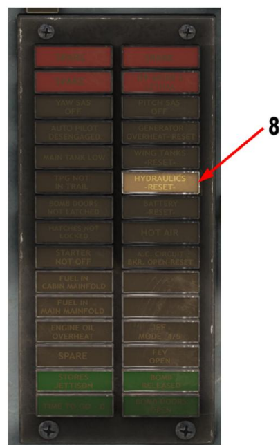
CENTRAL CAUTION PANEL
