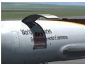
Main Cargo Door – Exterior Model
