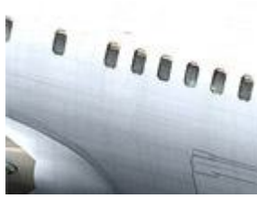
No Starboard Fwd Service Door
