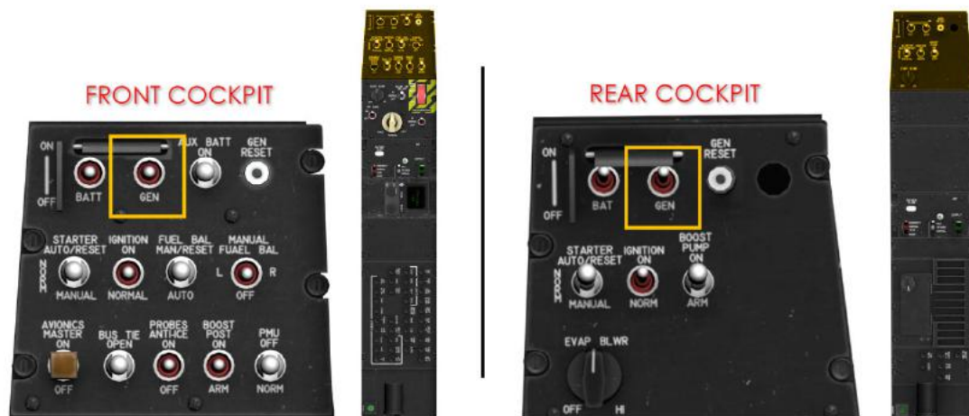
Figure 1-13 Generator Switch Location/s
