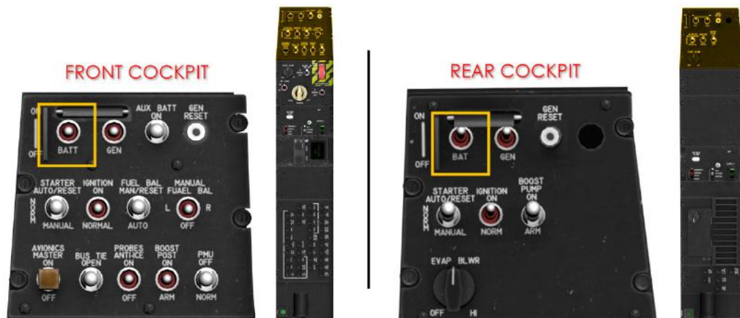
Figure 1-14 Battery Switch Location/s
