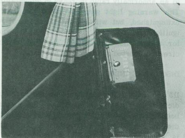
Figure 1-18 Cabin Door Hinge Emergency Release
