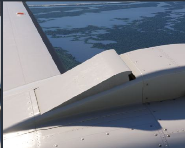
Right: partially extended - flight position
