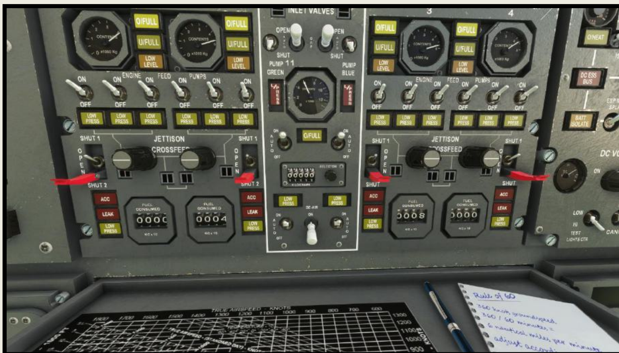
Engine Feed Pumps all ON, Low Pressure Valves OPEN ( red covers lowered ) and Jettison Crossfeed dials to IN-LINE ( black knobs with grey top and white lines ).
