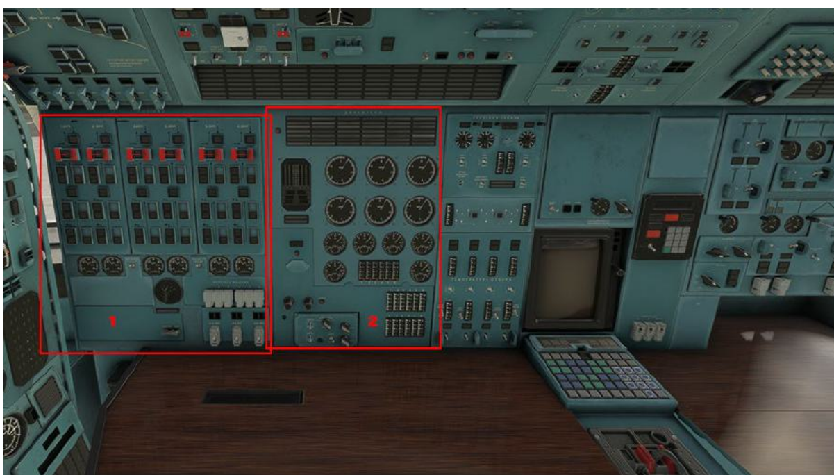
1. Fuel Panel (FO Side)
