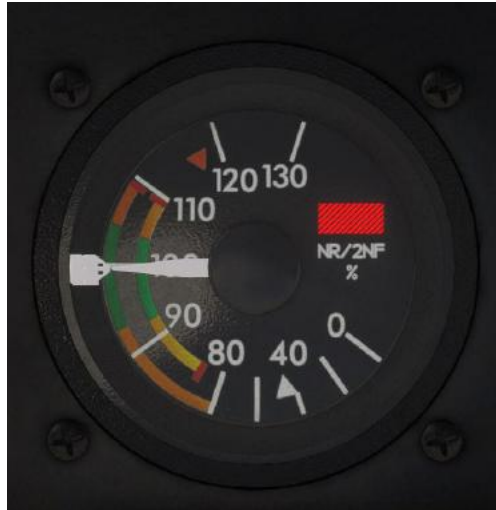
Triple RPM indicator (NR, N2 for each engine) with red failure flag
