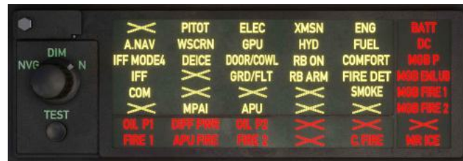
Warning Caution Panel (WCP)
