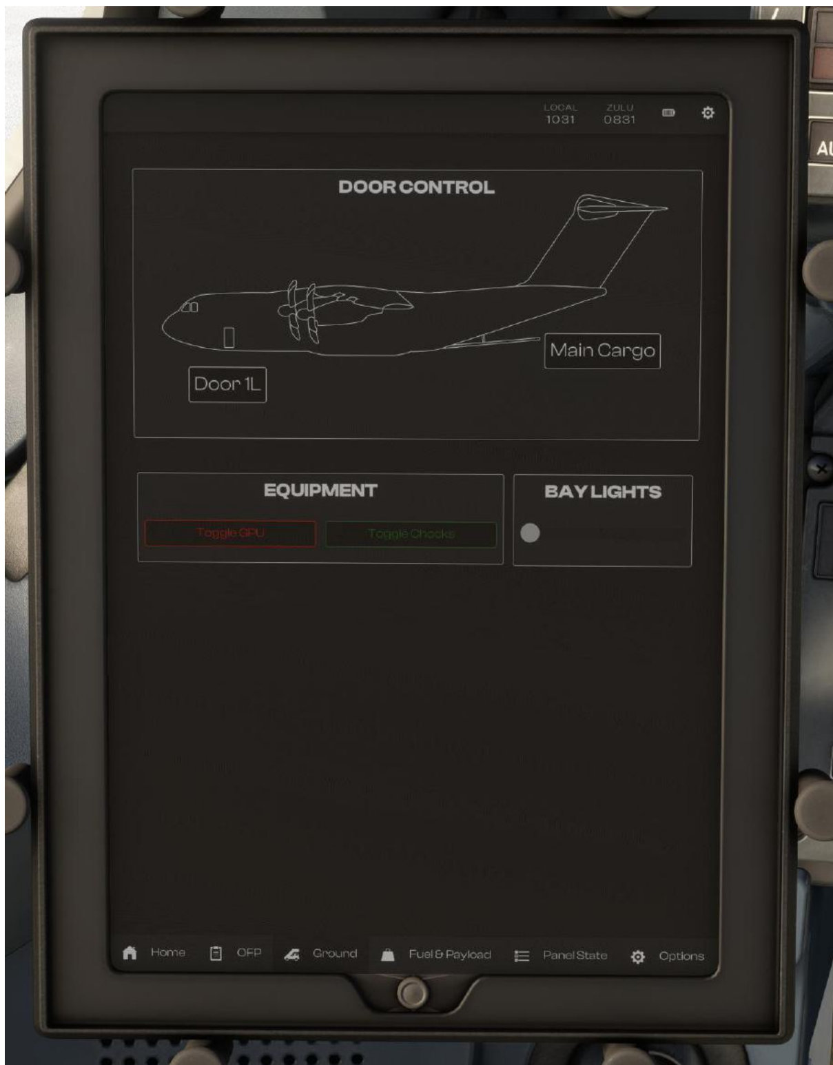
Ground Page – Controls doors on the aircraft along with requesting external Ground Power, chocks and illumination of the cargo bay.
