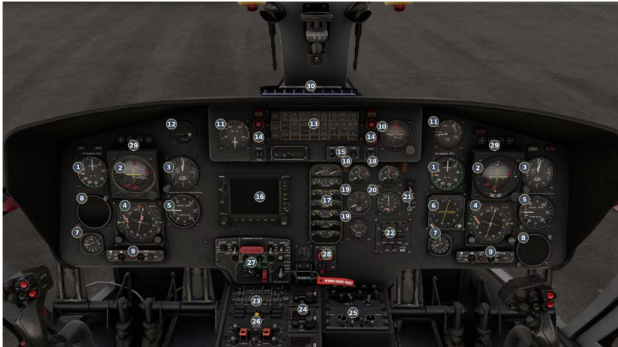
Figure 5-1 — AS365 N2 instrument panel (callout numbers refer to the instrument guide below)
