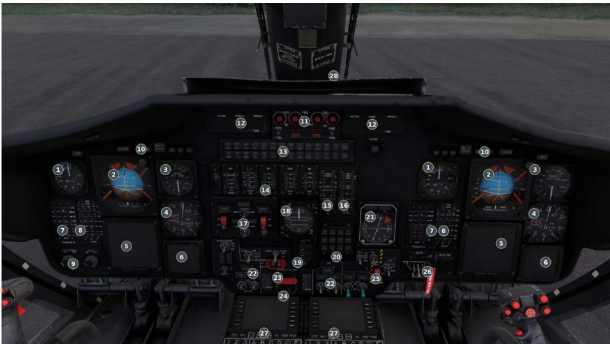
Figure 6-1 — HH-65A instrument panel (callout numbers refer to the instrument guide below)
