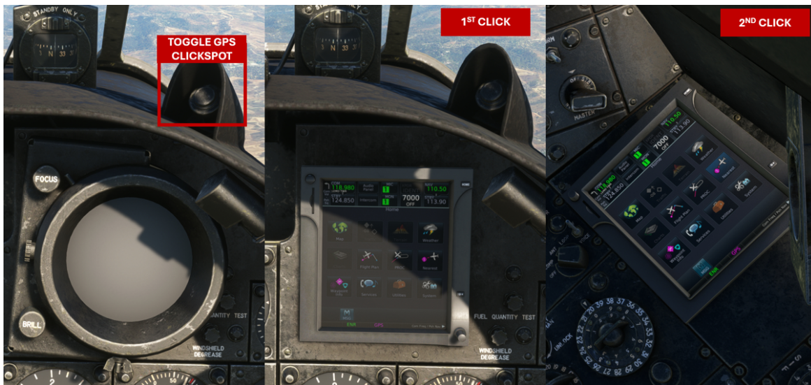
Location of the PMS GTN750 Navigation Unit; and Toggle GPS Clickspot
