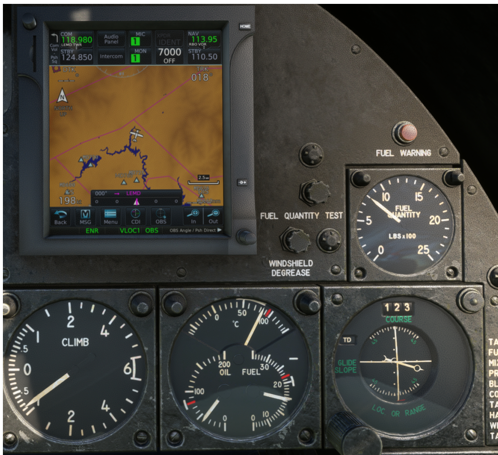
Course-Bearing/OBS Indicator on the bottom-right corner indicating direction of VOR Station
