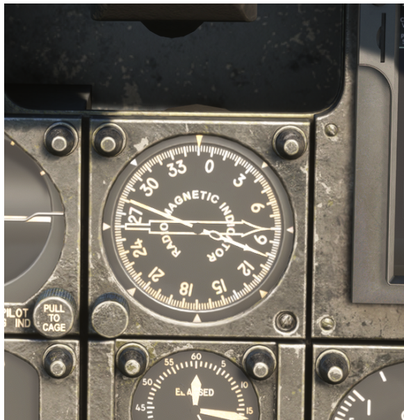
Small Needle displaying bearing to ADF.
