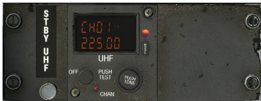
UHF Backup Control Unit
