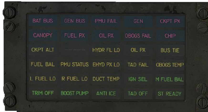
Master Caution and Fire Warning Annunciator
