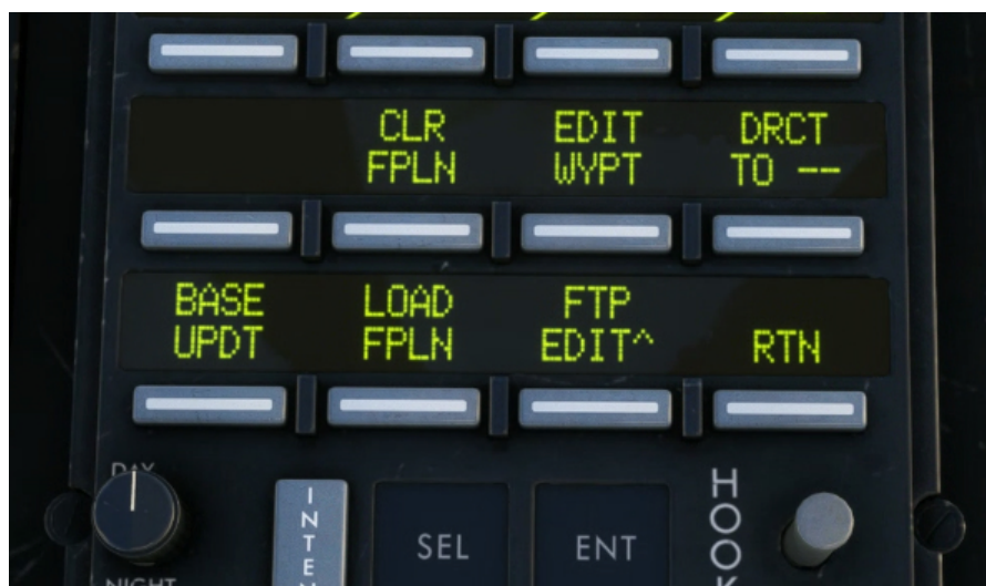
FTP Edit Submenu, displaying option CLR FPLN
