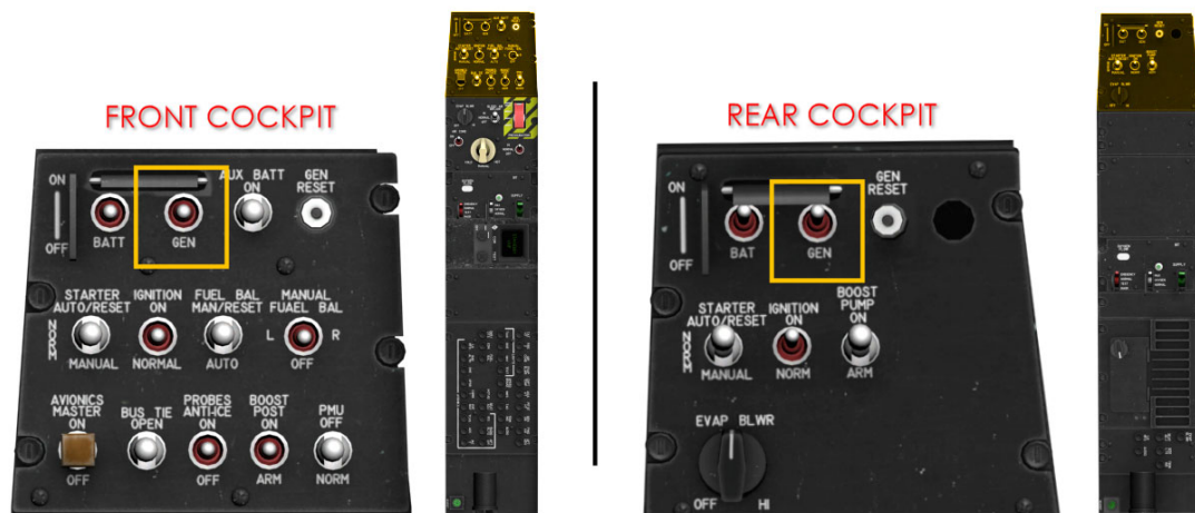
Figure 1-13 Generator Switch Location/s
