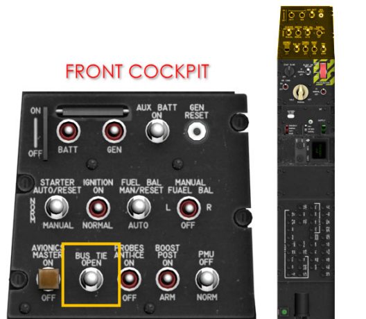
Figure 1-16 Bus Tie Switch Location
