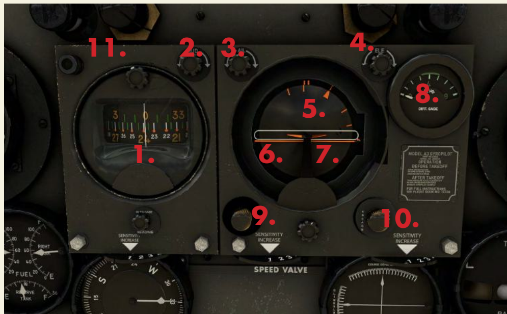
1. Index & Gyro cards 2. Heading Adjust 3. Bank Adjust 4. Pitch Adjust 5. Bank indicator 6. Pitch Reference (bug) 7. Pitch indicator 8. Suction Gauge 9. ON/OFF 10. Cage Knob 11. Illumination
