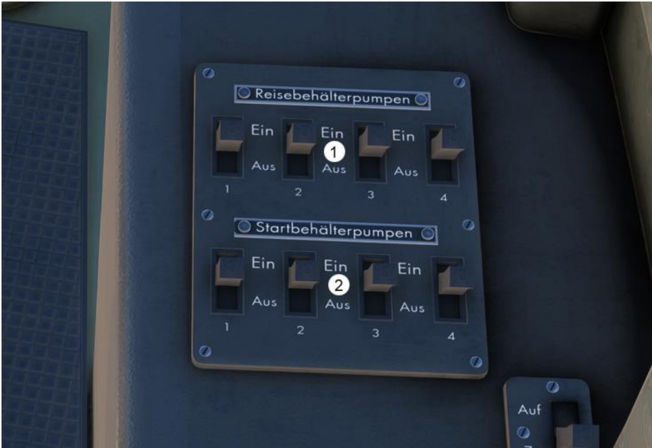
The fuel system pump panel is located on the left side of the copilot seat.
