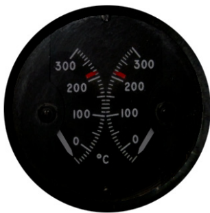
WING ANTI-ICING HEATER AIR TEMPERATURE INDICATOR
