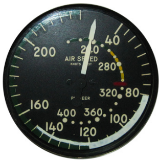
AIRSPEED INDICATOR (for 93,200 pound airplane)
