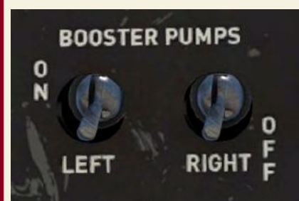
FUEL BOOSTER PUMPS... OFF
