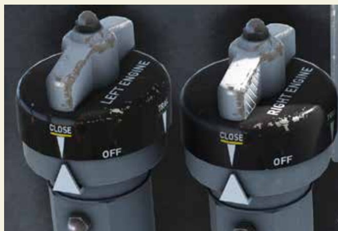
CLOSED POSITION; In this position the flaps are closed and lay flat against the body of the engine cowling.
