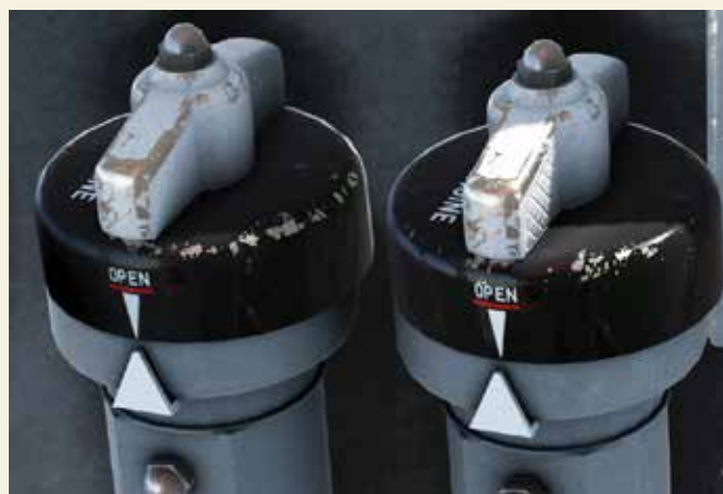
OPEN POSITION; In this position the flaps are fully open and remain so until another selection is made. ALWAYS use this position when engines are running on the ground.
