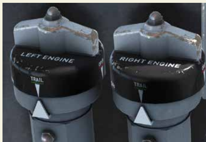
TRAIL POSITION; In this position, the flaps take up an angle dependent on airflow through the cowling. The faster the airflow, the flatter the flaps will lay. Slow speeds will open the flaps to aid engine cooling. This all happens automatically.
