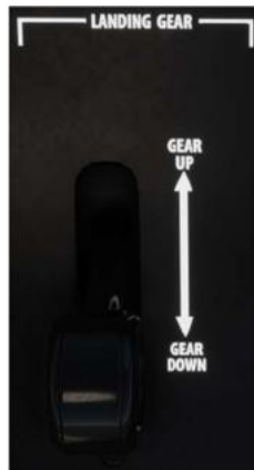
Fig 14-4-1 – Landing gear handle
