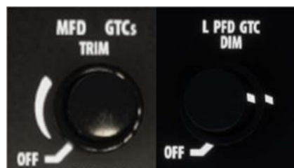
Fig 16-2-2 – Glass Cockpit Panel lighting knobs
