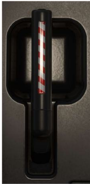
Fig 14-3-1 – Emergency/Parking brake handle
