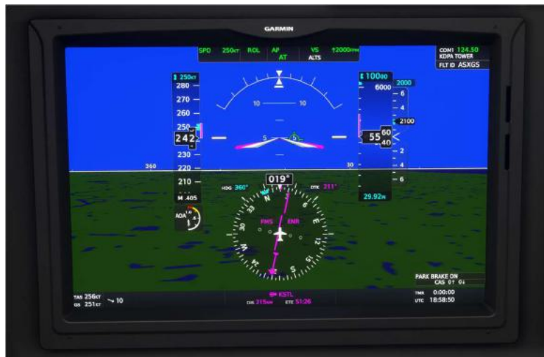
Fig 4-3-1 – The Primary Flight Display
