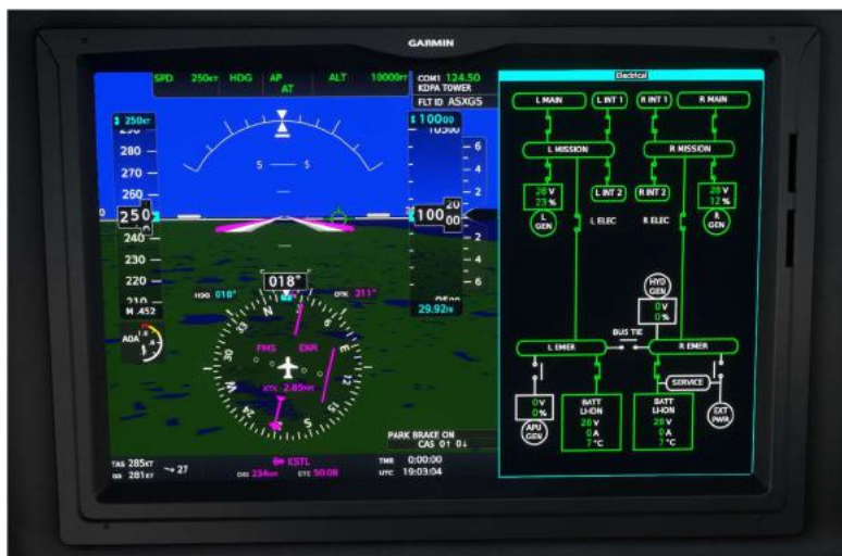
Fig 4-4-1 – The Primary Flight Display, in Split Mode
