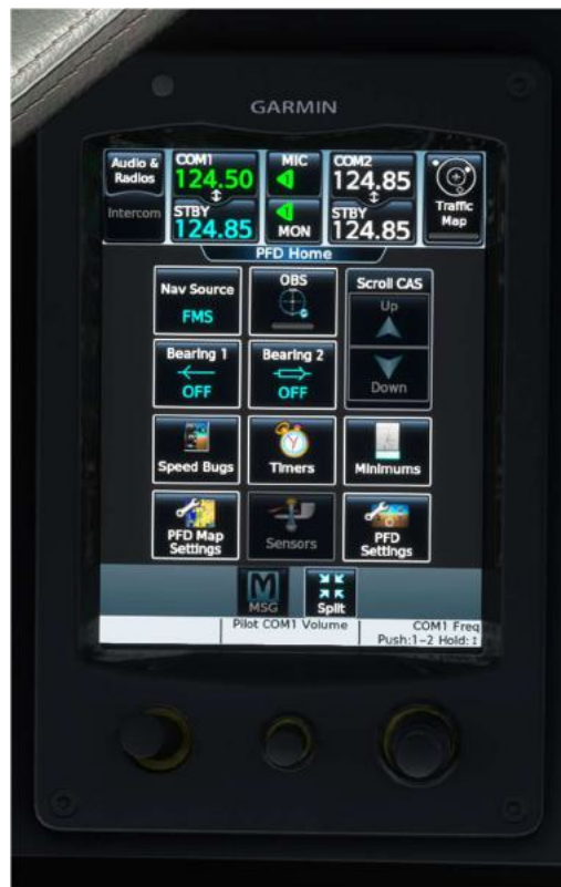
Fig 4-7-1 – The PFD Garmin Touch Controller
