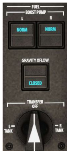
Fig 6-3-1 – Fuel System Controls
