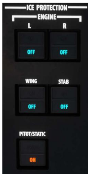
Fig 12-3-1 – Ice Protection Controls
