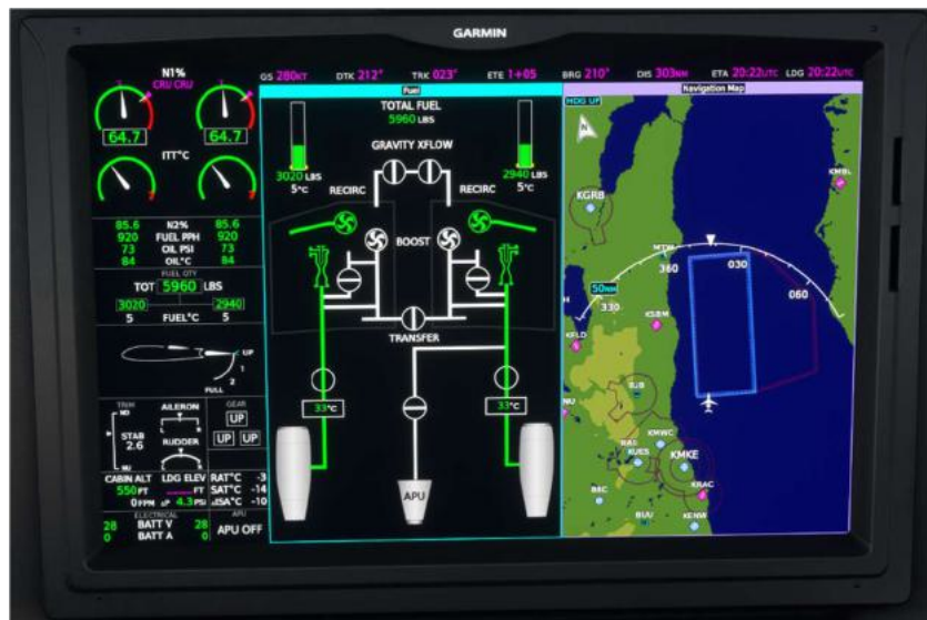
Fig 4-6-2 – Multi-Function Display in Split Pane Mode
