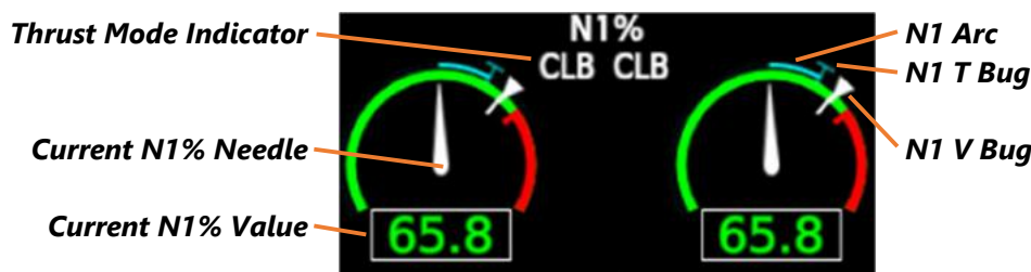
Fig 6-5-1 – EIS Engine N1 Indicators
