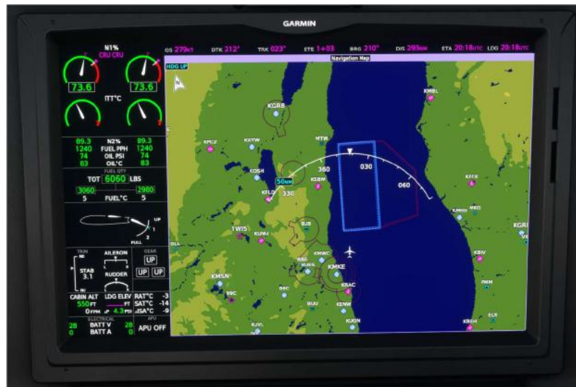
Fig 4-6-1 – Multi-Function Display in Full Screen Mode
