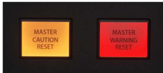
Fig 3-2-2 – Master Caution and Master Warning indicator/buttons
