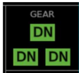
Fig 14-4-2 Landing gear indications
