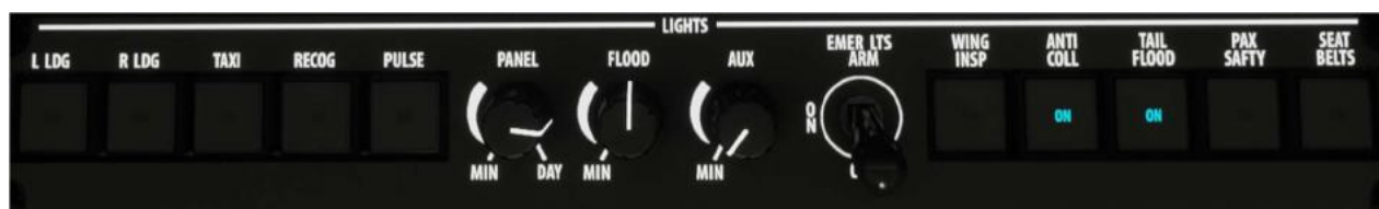
Fig 16-3-2 – Overhead lighting panel
