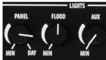
Fig 16-2-1 – Overhead cockpit lighting controls
