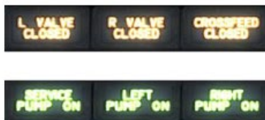
Figure 11-9. Annunciators Fuel Panel.
