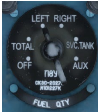
Figure 4-23. Fuel quantity switch.
