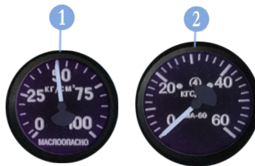
Figure 6-5. Air pressure gauges.
