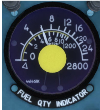
Figure 4-25. Fuel quantity indicator.
