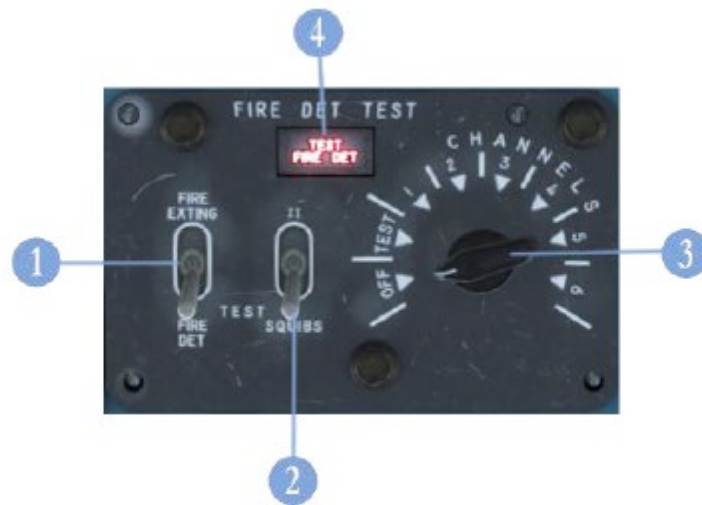
Figure 11-4. Fire Detection Test Panel.
