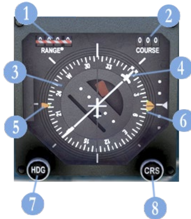
Figure 4-6. Horizontal Situation Indicator
