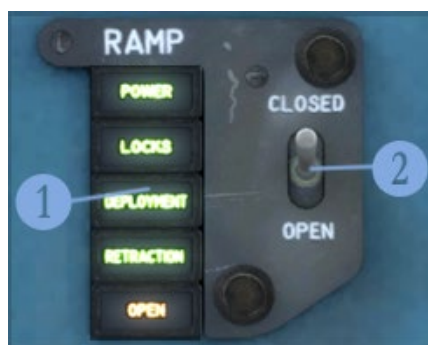
Figure 5-5. Ramp control panel.
