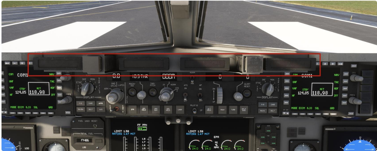
Fire Extinguisher Handles
