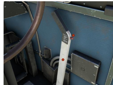
Figure 10-2: Manual gear lever. (1) Select mode: raise or lower (2) operate the ratchet mechanism.
