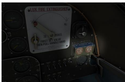
Figure 11-4: Feathering buttons for both engines are located on the far right side of the instrument panel.
