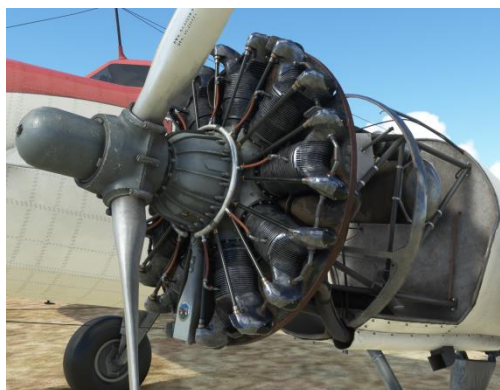
Figure 11-1: The Pratt & Whitney Wasp S1H1-G radial engine.
