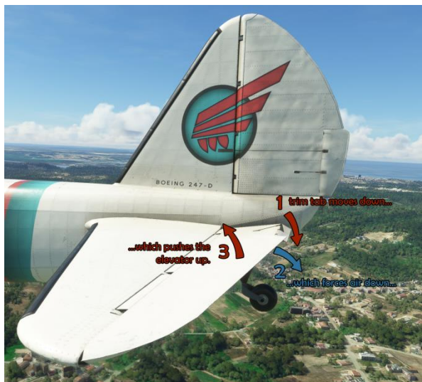
Figure 9-2: Forces induced by the trim tab.
