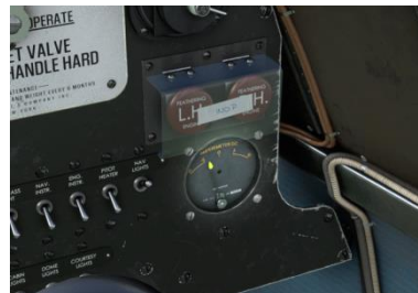
Figure 14-3: The ammeter shows a negative current, the battery is discharging.
