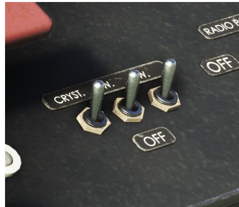
Figure 17-1: The three obsolete crystal switches.
