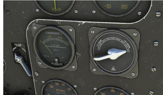
Figure 11-2: Engine temperature gauge to monitor cylinder head temperatures and carburetor temperatures.
