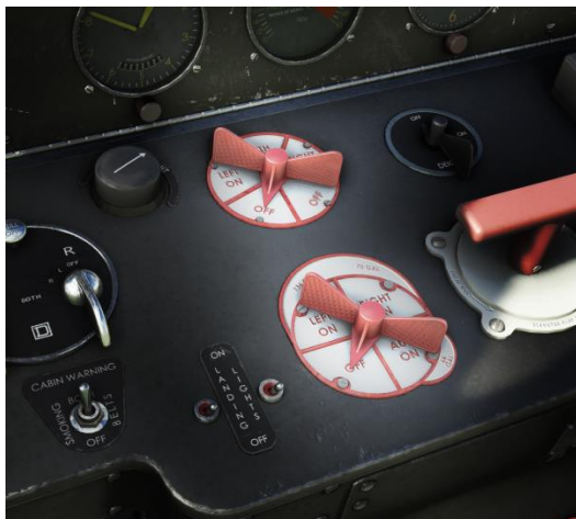
Figure 13-1: Top - engine distribution dial. Bottom - fuel tank distribution dial.
