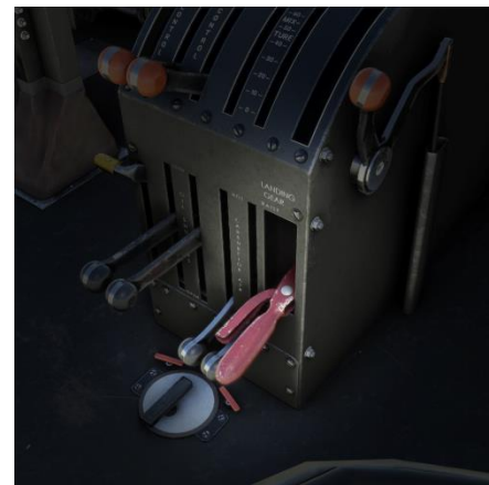
Figure 10-1: Location of the gear lever.
