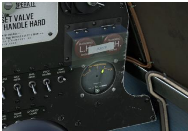
Figure 14-2: The ammeter shows a positive current, the battery is recharging.
