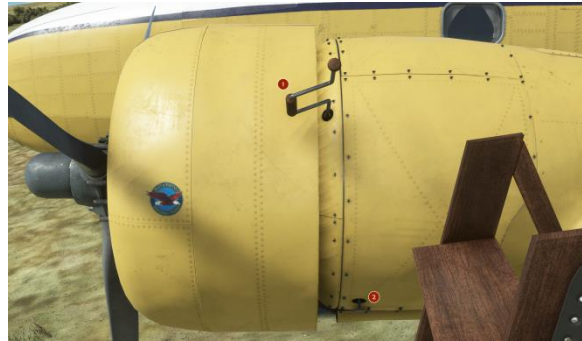
Figure 8-2: Controls for the manual start. (1) Starter crank. (2) Starter clutch.
