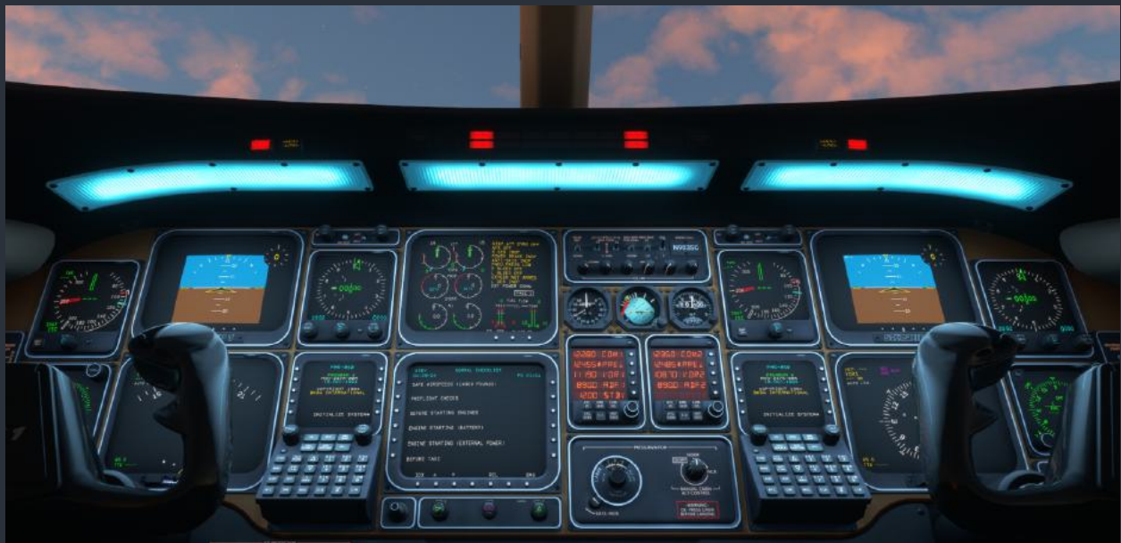
Glareshield electroluminescent lighting
