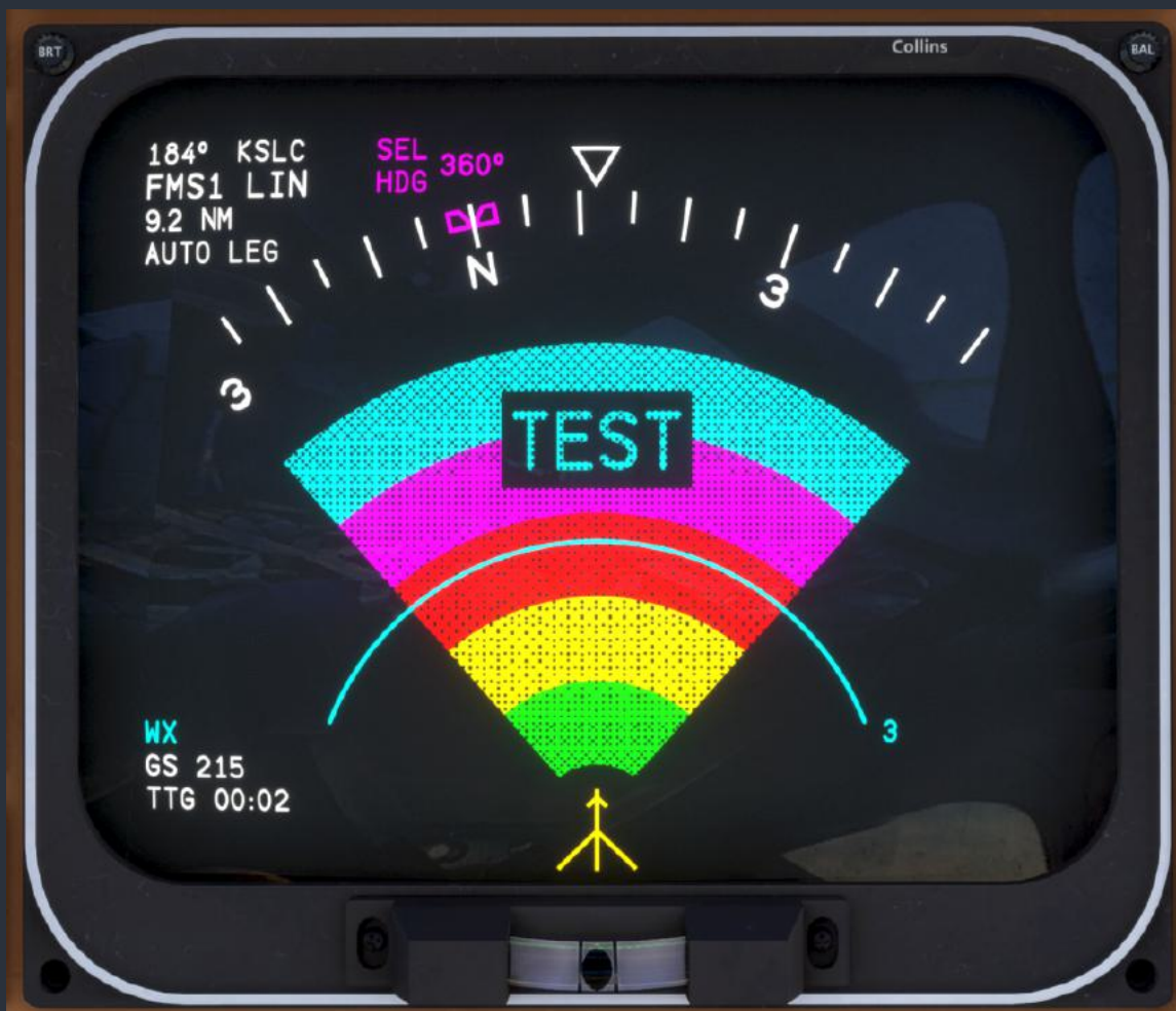
Radar test pattern on ND ARC display
