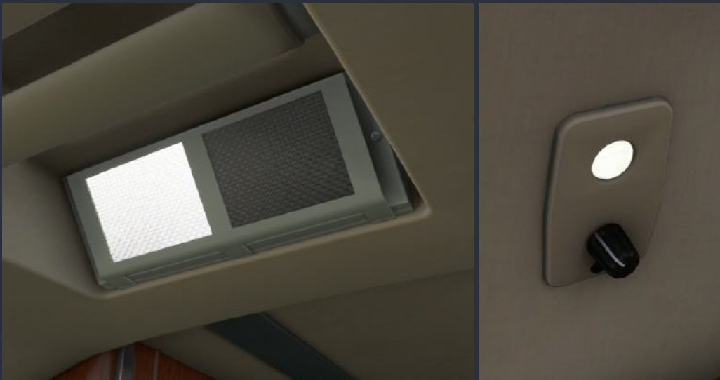
Storm flood light “LOW” (left), and pilot’s map reading light (right)
