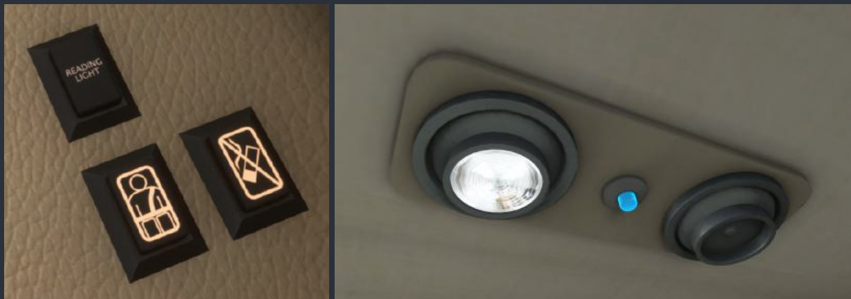
Individual passenger reading lights switch, seatbelt & no smoking sign (left), and lavatory lighting fixtures (right)
