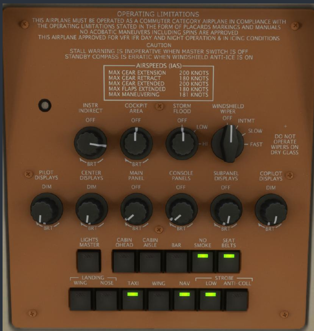
Overhead lighting control panel
