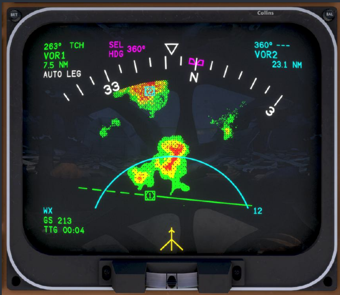
Weather radar with VOR active course
