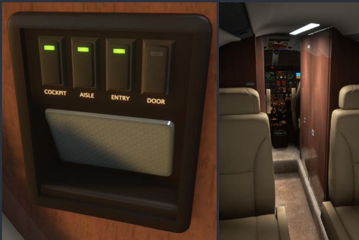
Cabin entry lighting control panel (left), and fluorescent cabin vestibule entry lighting (right)
