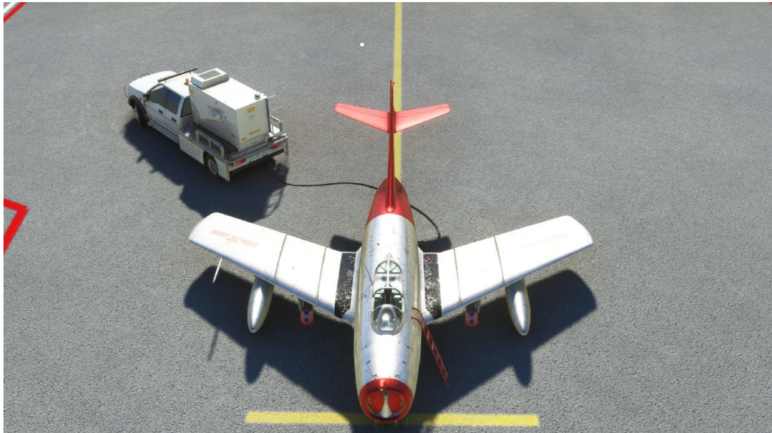
Fig 4-1 Ladder, Wheel Chocks and GPU connected on Ground
