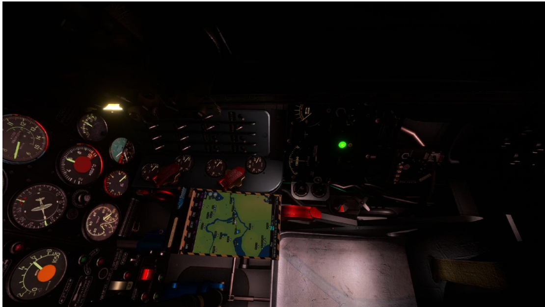
Fig. 0-14 Right Flood Light, AKR-7 Gauge Light, with Potentiometer Dimmer Controls
