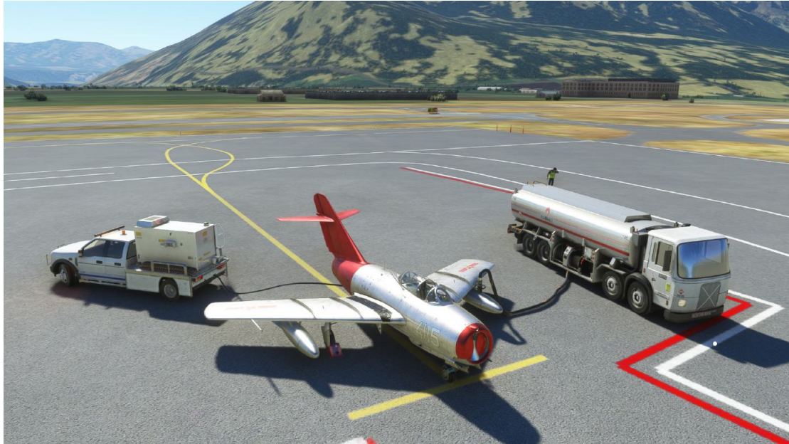
Fig 4-2 Fuel Truck and GPU connected on Ground
