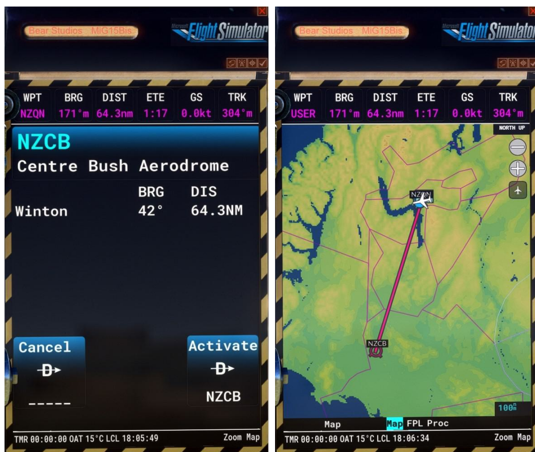
Fig 15-1 AS3X Touch GPS Direct To Input Pages
