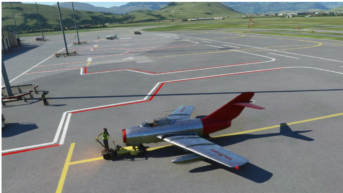
Fig 4-3 Pushback Tug connected on Ground
