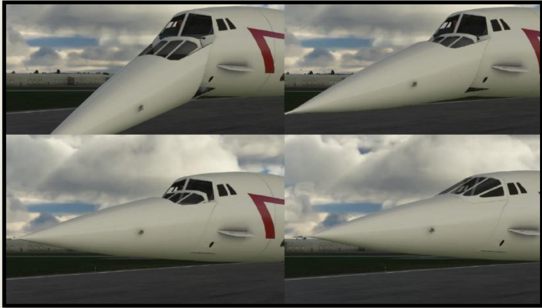
The four stages of Concorde's variable nose geometry, from top left:
