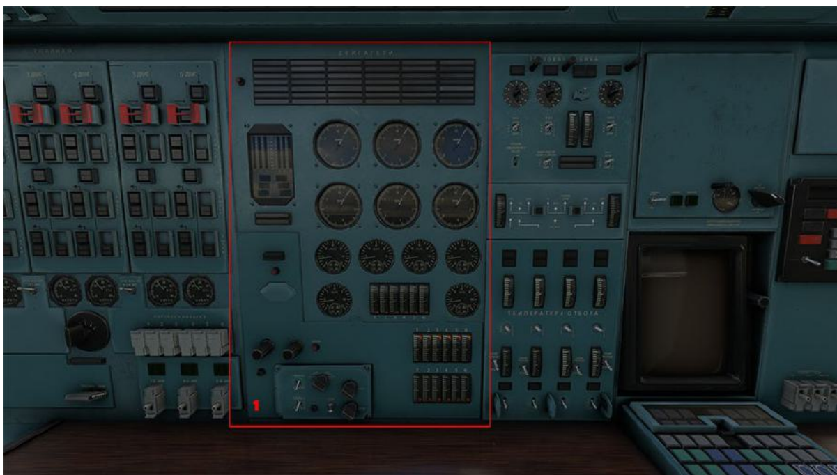
1. Engine Panel (FO Side)
