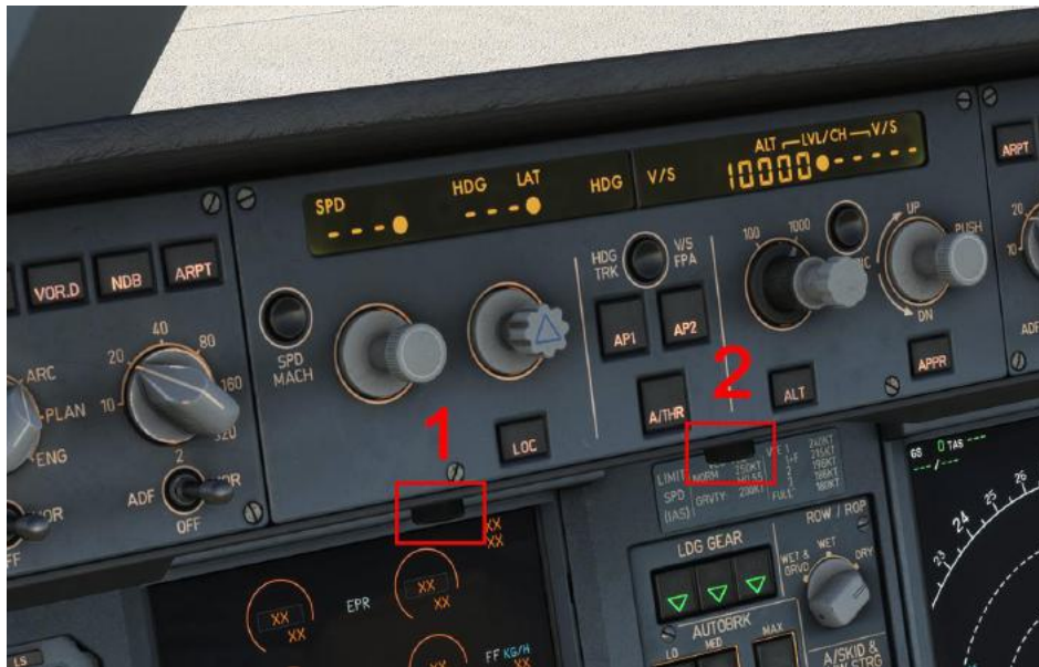
1. Glareshield Integral Lighting knob
