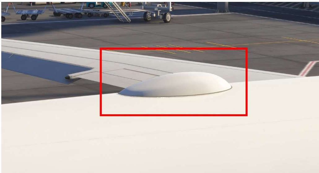
SATCOM – Satellite communications antenna, located on the aft upper fuselage.
