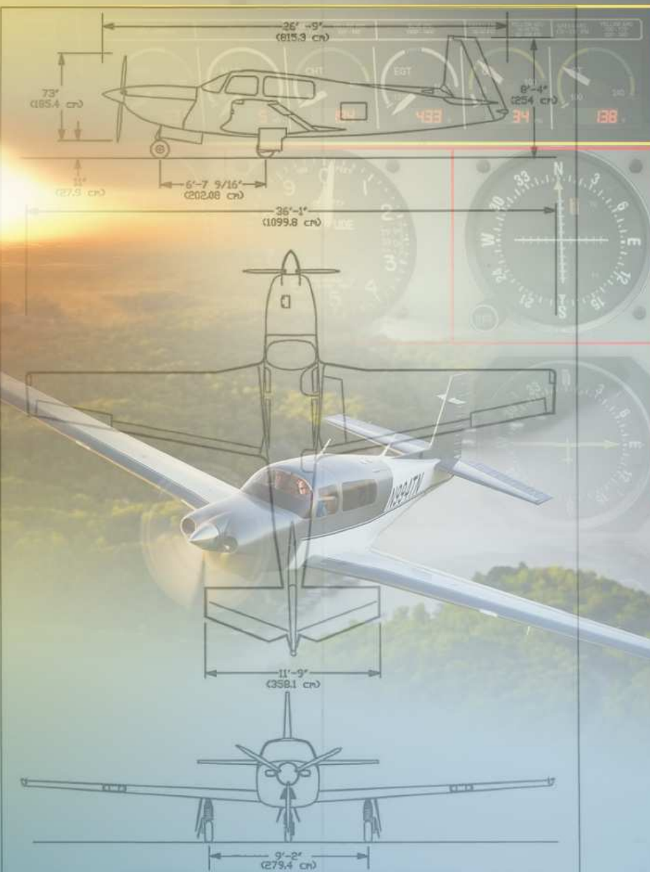
FIGURE 1 - 1 THREE VIEW - M20R
